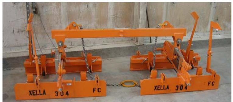
**Figure 5B.5: Floor and Roof Panel Lifting Gear**
