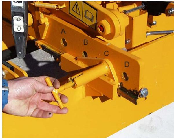
**Figure 5B.13: Pulling Pin to Position Clamping Jaw**
