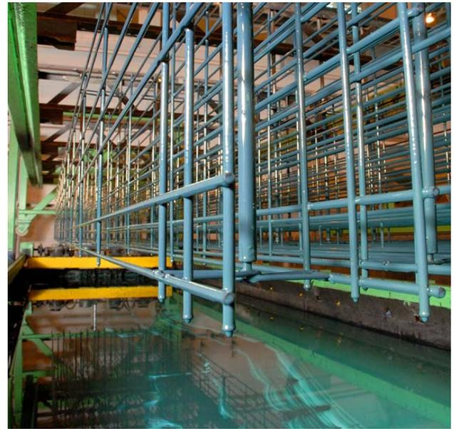
**Figure 1.8: Anticorrosive Agent Application to Reinforcing Wires**
