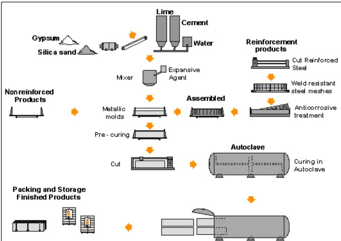
Figure 1.5: Diagram of Hebel AAC Production Process
