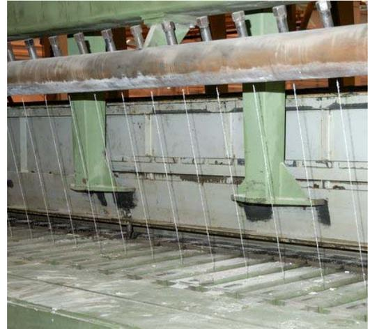
Figure 1.4: Cutting Machine with steel wires
